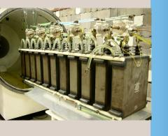
**Above image, top:** HELCAT (HELicon-CAThode) 4-meter-long basic plasma physics research device at the UNM Plasma & Fusion Science Lab. **Above center:** 500 kV Marx generator at the UNM Pulsed Power, Beams & Microwaves Lab. **Below:** Low-inductance oil switch designed to generate a high-voltage pulse with sharp risetime on the Marx generator above.
