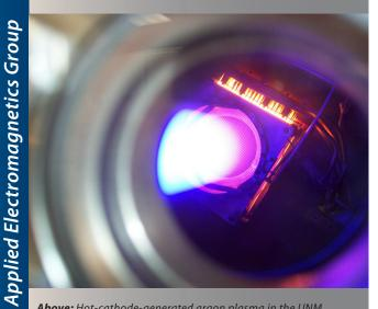
**Above:** Hot-cathode-generated argon plasma in the UNM Plasma & Fusion Science Lab. **Below:** A "transparent cathode" invented at UNM is used to drive high-power magnetrons with greatly enhanced performance.
