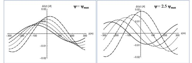
Figure 3. Current waveform spread at  $\psi = \psi_{max}$  vs. larger  $\psi$
